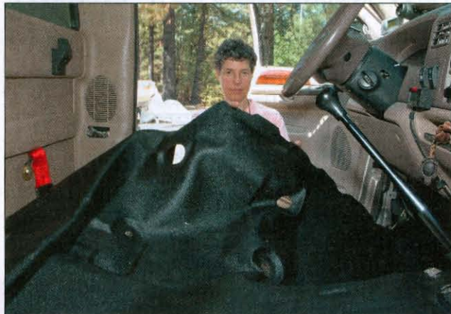
We needed to cover the Dynamat and Heat Shield insulation so we ordered a rubber floor mat from our local Ford dealership. The factory mat was a pretty good fit, but we still had to do some custom cutting around the transfer case lever and the rear wall.
