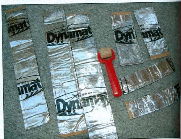
Each Acoustishield hood kit comes with a pre-cut selection of Dynamat strips. A full Dynamat kit would use much more material and be far more expensive.
