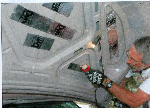
Peeling off the backing of the Dynamat, each strip was placed on the single-wall sections of the hood and pressed with a wallpaper seam roller for maximum surface contact.
