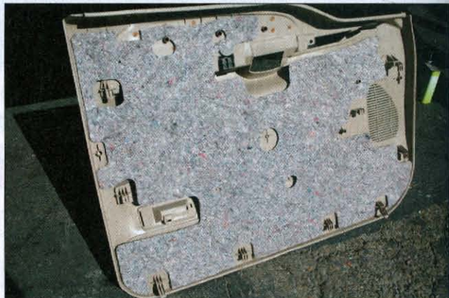
The factory Super Duty door panels came padded with this sheet of insulation. Ours were still in very good shape, but if you live in a wet climate, this material may be damaged to the point that you can't reuse it. The same goes for the plastic dust cover material that lines the door shells.
