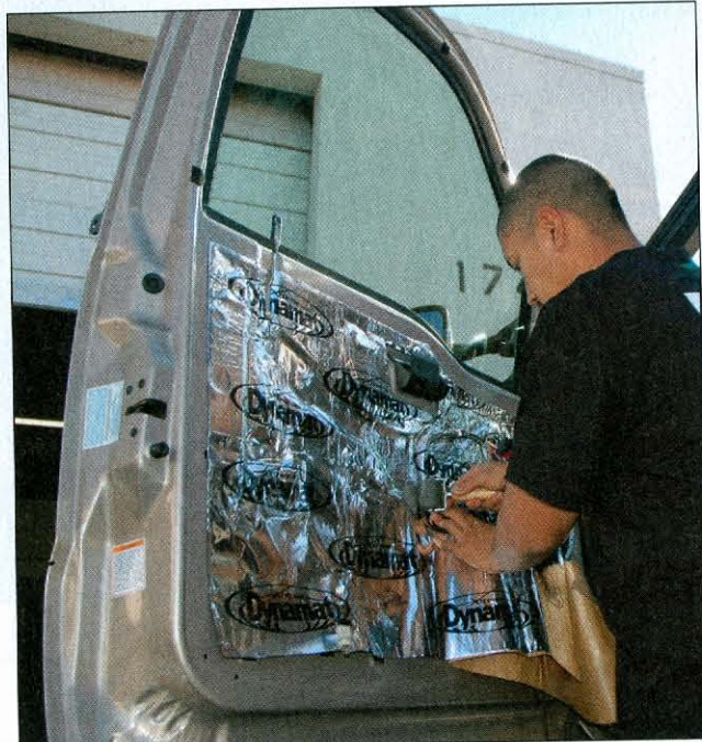
Full sheets of Dynamat were applied to both the inside and the outside of the doors for maximum noise reduction.
